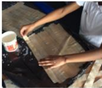
Step 4: Lay the strips side by side, overlapping them slightly.
